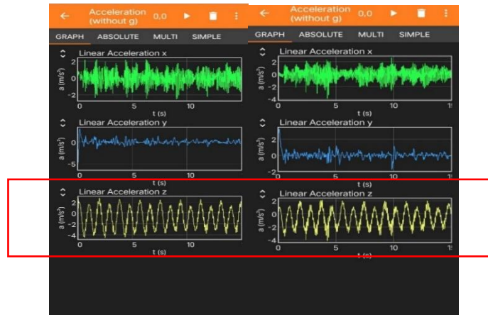
Figure 3. Smartphone sensor data results showing oscillation period
