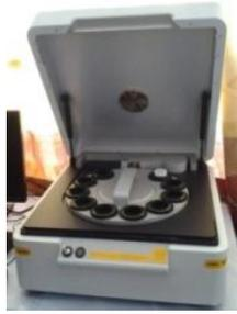
Gambar 7. X-Ray Fluorescence Spectrometer (PANanalytical type Epsilon 3)
