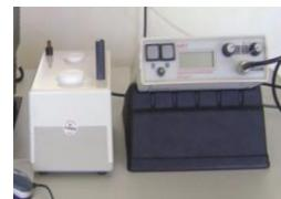
Gambar 5. *Magnetic Susceptibilitymeter* (*Bartington Susceptibilitymeter type MS2*)
