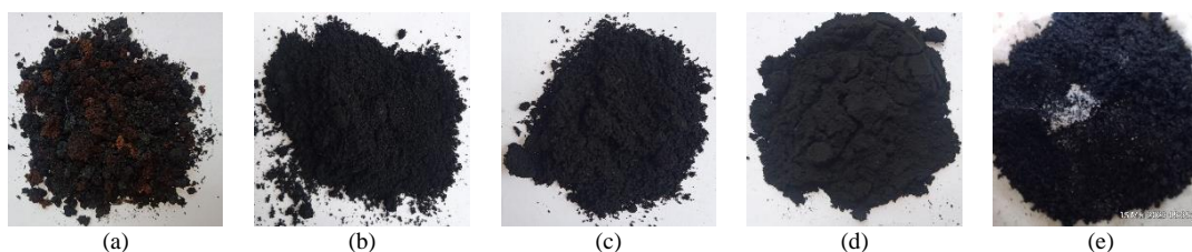
Fig. 2. Results of coconut pulp carbonization at temperature (a) 250°C, (b) 300°C, (c) 350°C, (d) 400°C, (e) 450 °C
