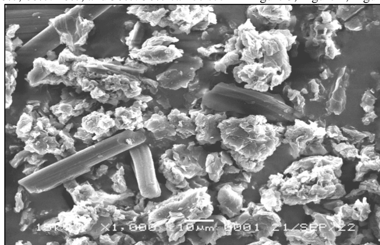
Fig. 3. Surface image of Graphene Oxide composition of 100% graphite composition with 1000X magnification
