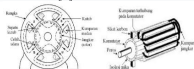
Fig 3. Contruction of direct current motor part stator (a) dan rotor (b) [6]
