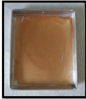
Fig. 3. Avocado seed starch biodegradable plastic.
