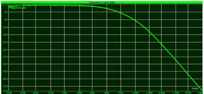
Fig. 5. Simulated frequency response of the low-pass filter circuit.
