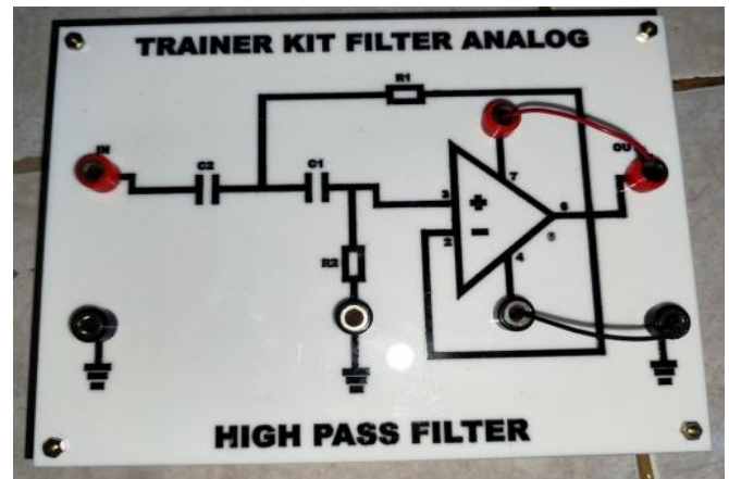
Fig. 2. Physical dimension and panel layout of the analog filter trainer kit.
