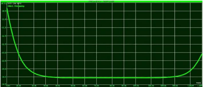
Fig. 8. Simulated frequency response of the band-stop filter circuit.
