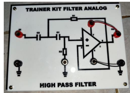
Fig. 3. Front view of the LM741-based analog filter trainer kit.
