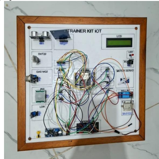
Fig. 6. Final appearance of the ESP32-based IoT trainer kit.
