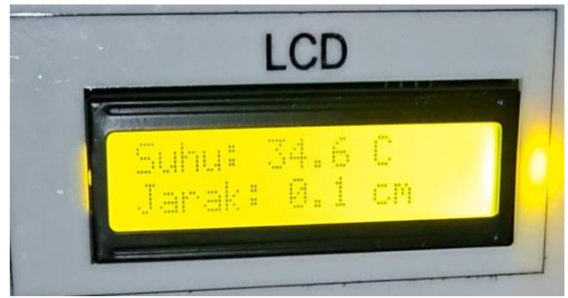
Fig. 8. LCD display of DHT22 and ultrasonic sensor readings.
