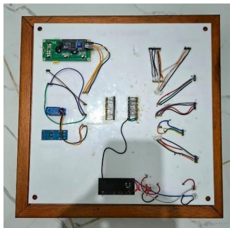
Fig. 5. Component wiring on the rear side of the trainer kit.
