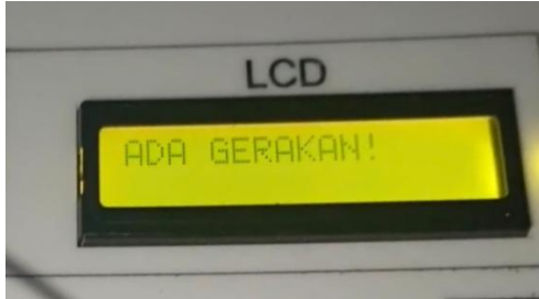
Fig. 9. LCD display when motion is detected by the PIR sensor.
