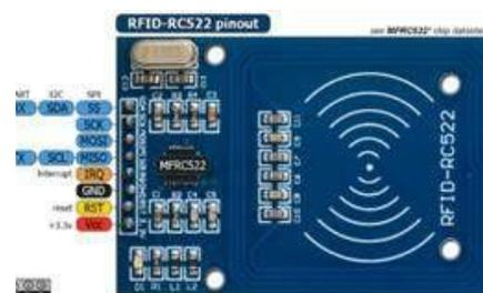
Gambar 2. RFID-RC522 pinout
