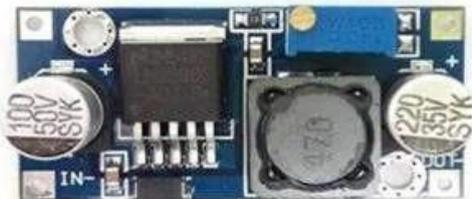
Gambar 5. Modul Step Down DC LM2596
