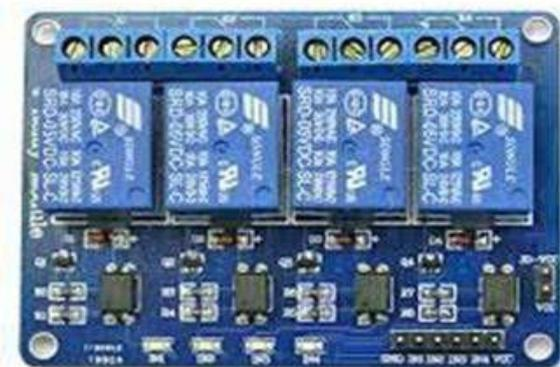
Gambar 6. Modul Relay 4 Channel
