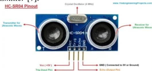
Gambar 3. Sensor Ultrasonik
