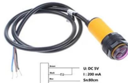
Gambar 3. Photoelectric Proximity Sensor
