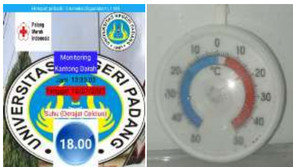
Gambar 8. Uji keakuratan sensor DHT11
