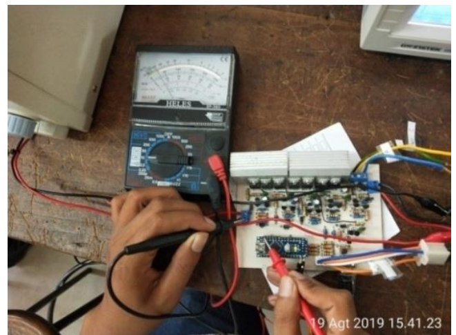
Gambar 15. Proses Pengukuran Driver Mosfet
