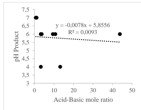
**Figure 3.** The Relationship Between The Acid-Basic Molar Ratio and The pH of The Output Water Product
