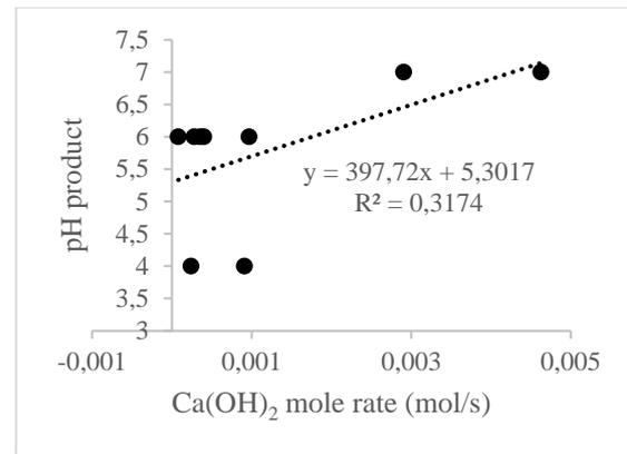
**Figure 2.** The Relationship Between Molar Flow Rate of  $Ca(OH)_2$  and The pH of The Output Water Product
