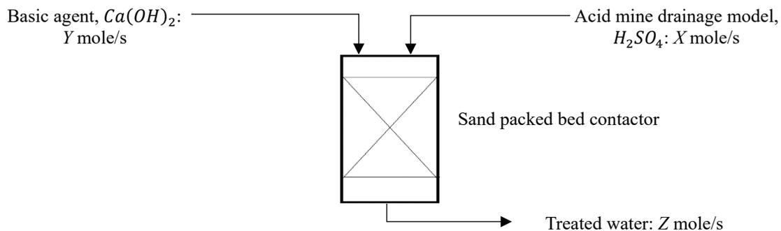
**Figure 1.** Schematic Model of Sand Packed Bed for Acid Mine Drainage Neutralization
