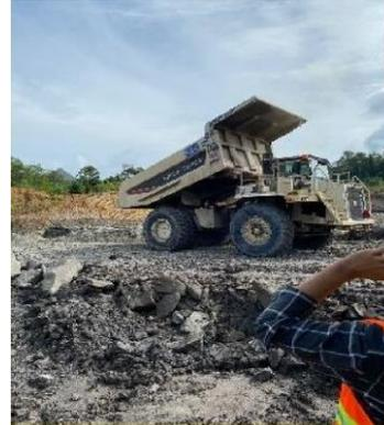
Gambar 5. *Dump Truck* Terex TR50D
