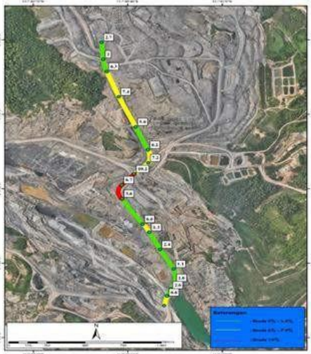
Picture 3. Road Grade Segment
