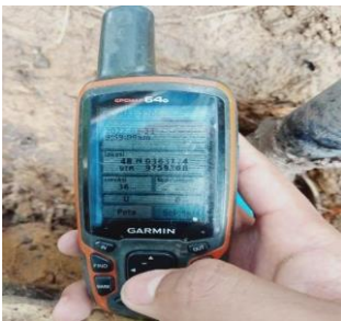
Fig 4. Retrieval of Coal Outcrop Coordinate Data and Dip Position using Garmin GPS
