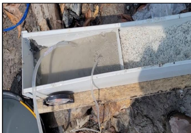
Figure 9. AMD pH Neutralization Testing
