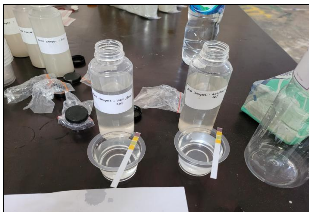
Figure 8. AMD pH Value Measurement
