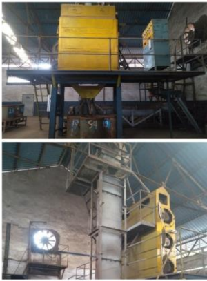
Gambar 6. High Tension Roll Separator di Amang Plant
