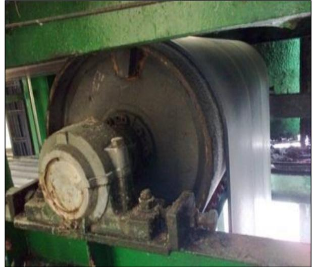
**Gambar 7.** Bend Pulley
