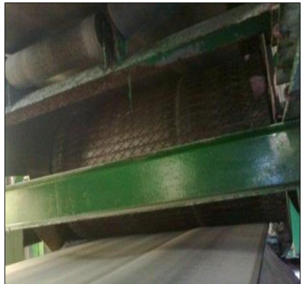
**Gambar 8.** Head Pulley
