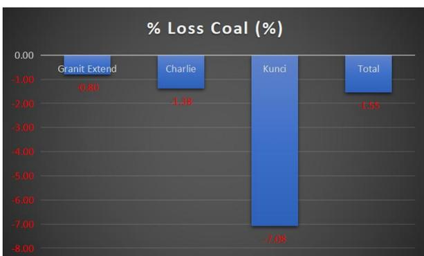
Gambar 11. Grafik *Coal Losses* di *StockROM Port*
