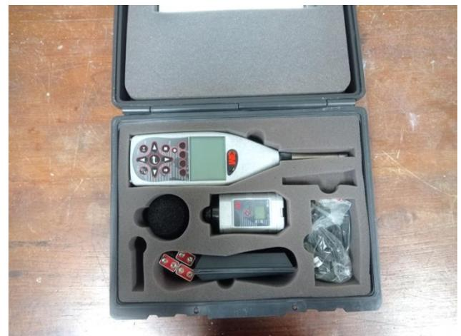
**Gambar 5.** Sound Level Meter Digital
