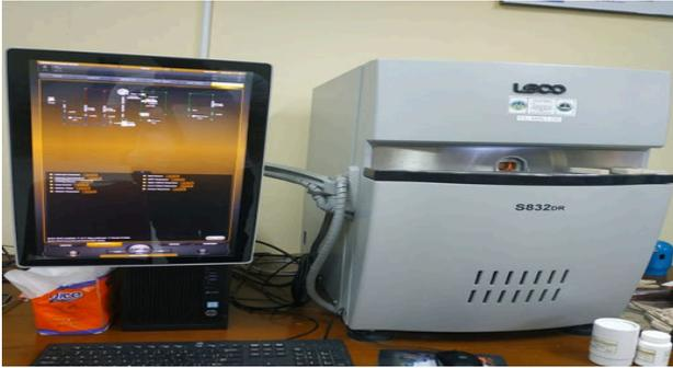
**Gambar 24.** Alat pengujian kadar sulfur batubara
