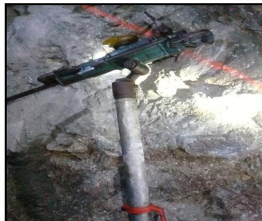
**Gambar 6.** Mesin Bor jack Leg
