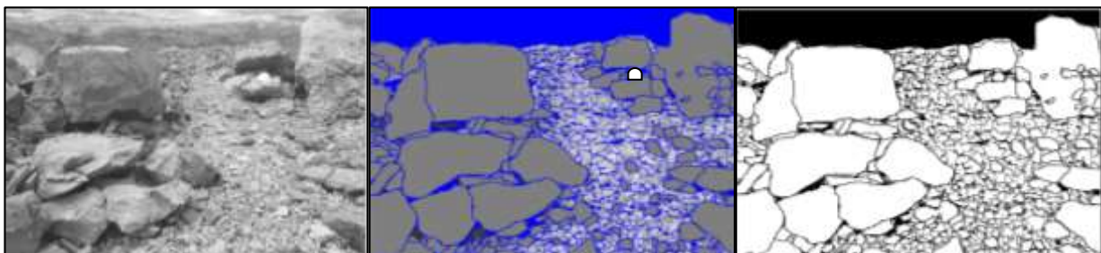
Gambar 2. Contoh pengukuran image analysis split desktop
