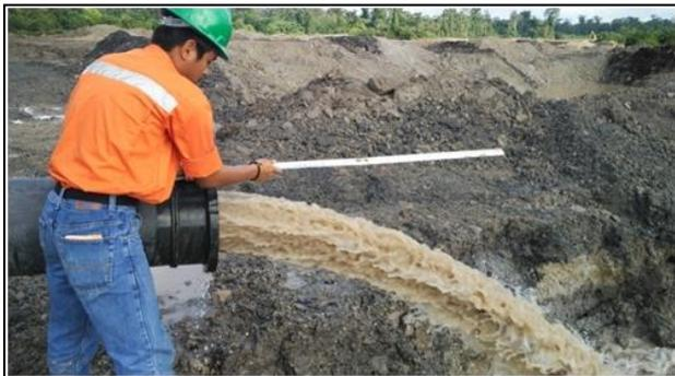
Gambar 5. Pengambilan Data Debit Aktual Pompa MF420 No Unit 7107 Main Sump A2
