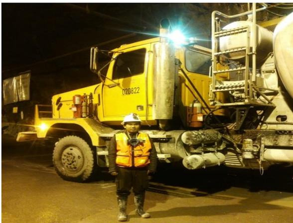
Gambar 3. Alat Angkut *Shotcrete* Mixer Truck
