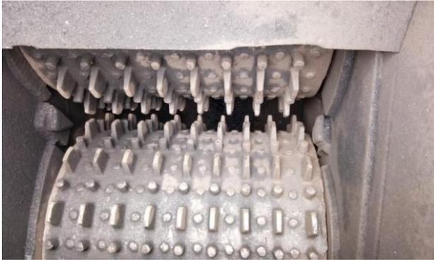
Gambar 7. Double Roll Crusher
