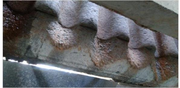
**Gambar 14.** Liner Jaw Crusher Bagian Bawah Sebelum Dibalikkan
