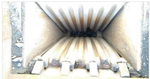
**Gambar 15.** Liner Jaw Crusher Bagian Atas Sebelum Dibalikkan
