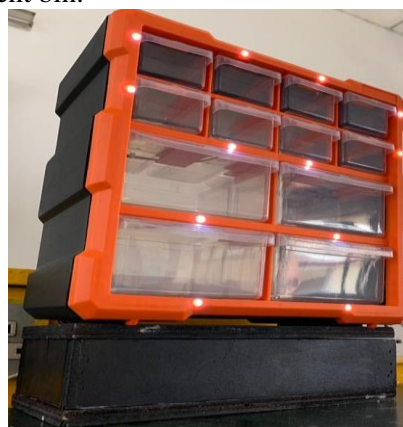
Figure 4 . Location of LEDs on a sample component storage bin
