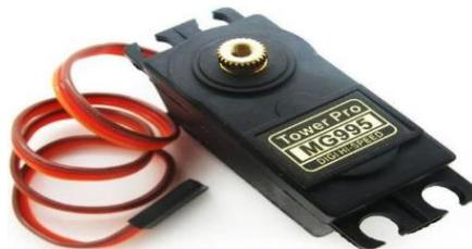
Gambar 4. Motor Servo MG995
