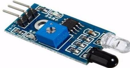
Gambar 3. Sensor Infrared
