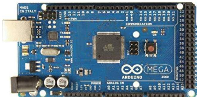
Gambar 2. Arduino Mega 2560
