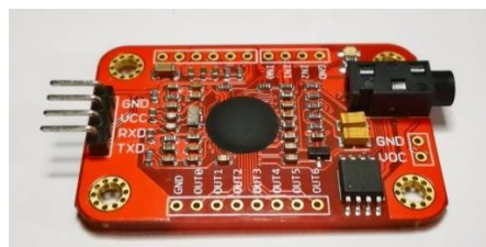
Gambar 1. Modul Voice Recognition V3
