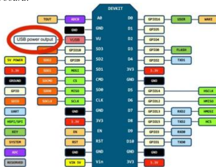
Gambar 1. Pin mapping NodeMCU ESP8266
