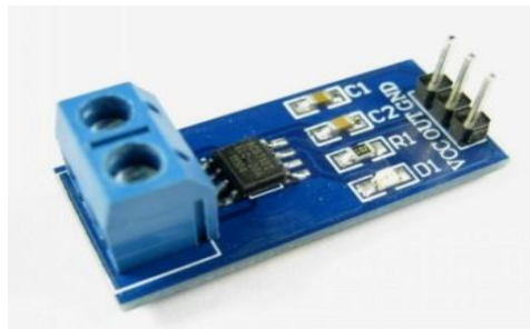
Gambar 8. Sensor Arus ACS712
