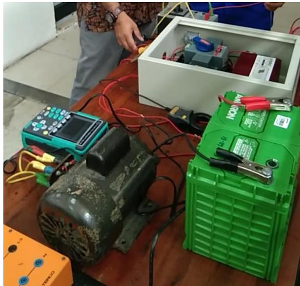
Gambar 4. Pengujian system hybrid Panel Surya – PLN beban motor
