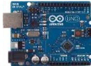
Gambar 3. Modul Arduino Uno [3].
