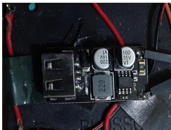
Gambar 4. Boost step up / down + USB port
