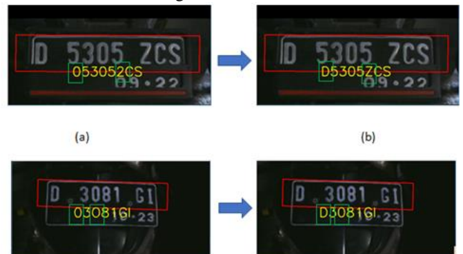
Fig. 14 The results of the character improvement process. Tests on the ANPR system were carried out on 100 previously prepared images. Of the 100 images, 98 images can be identified. Where the use of character improvement algorithms can increase the recognition that initially only 84
