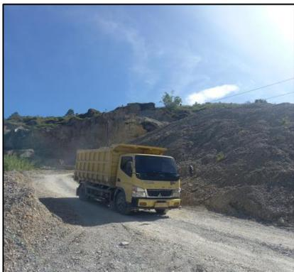
Gambar 5. Dump truck Colt Diesel Canter SHdx (14 Ton)
