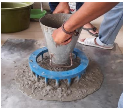
Gambar 1. Uji J-Ring Tester
