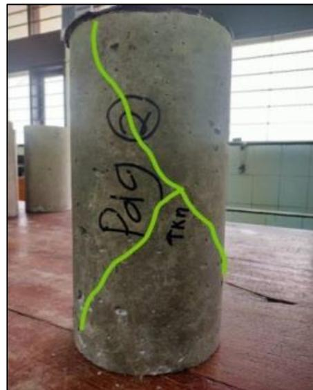
Gambar 13. Pola Retak *Cone and Shear* Beton Pasir Padang
