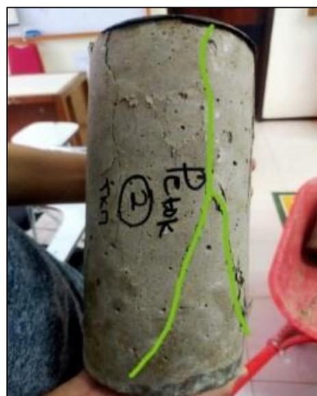
Gambar 14. Pola Retak *Cone and Split* Beton Pasir Petok
