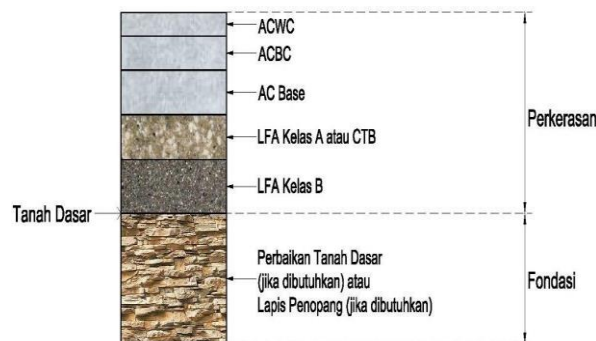
Gambar 2. Struktur Perkerasan Lentur (Flexible Pavement) [5]
