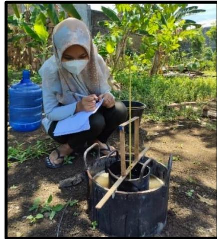
Gambar 1. *Double Ring Infiltrometer*
