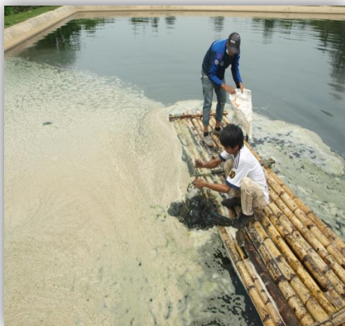
Gambar 2. Proses Pengambilan Sampel Lindi di Kolam Lindi
