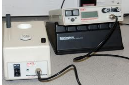
Gambar 4. Bartington Susceptibility Meter Tipe MS2
