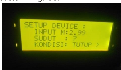
Fig 5. Display of Angle Reading on LCD
